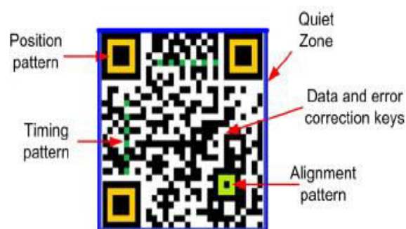
Fig. 2. Structure of QR Code
