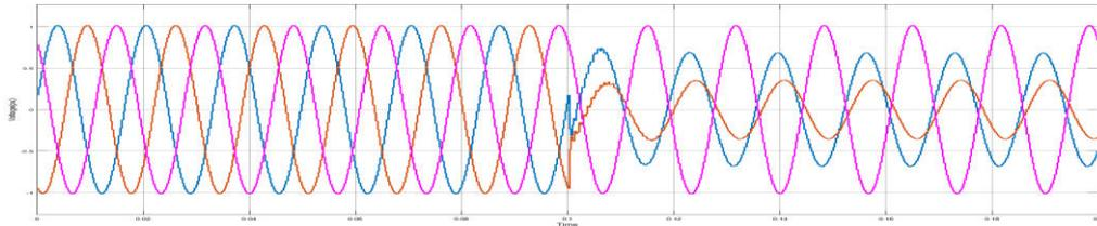
Fig.3(d). Voltage waveform of L-L (A-B) fault
