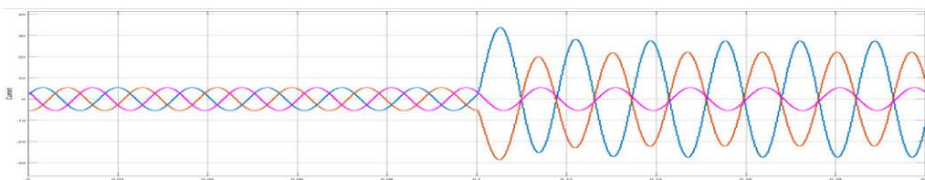
Fig.3(c). Current waveform of L-L (A-B) fault
