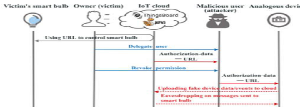
Fig. 5. Flaw 4 — URL leakage in ThingsBoard and Kaa Enterprise.
