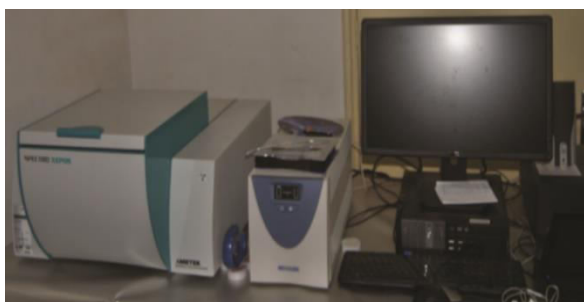
Fig 1: Overview of the SPECTRO XEPOS X-ray Fluorescence Spectrometer
