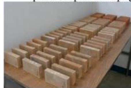
b) Selected sample bricks in vertical position to prevent warping
