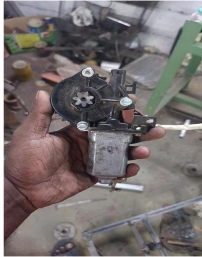
Fig.5 (b) illustrates the Rotation of upper chassis to desired angle using high-torque motor
