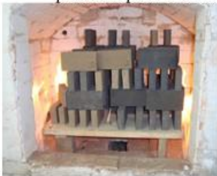
c) Distribution of selected sample bricks inside the kiln to ensure even burning
