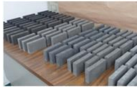
b) Selected sample bricks in vertical position to prevent warping
