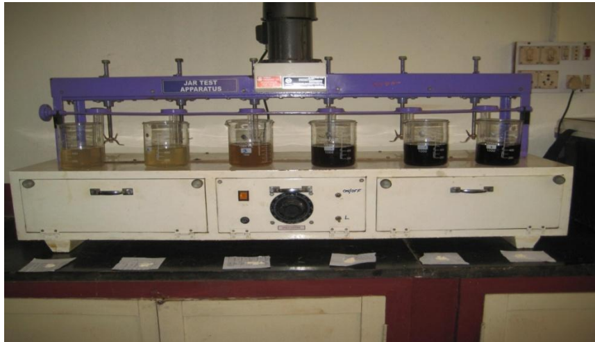
Fig 2.5: A conventional jar test apparatus
