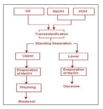
Fig 1. Flow chart of production of biodiesel
