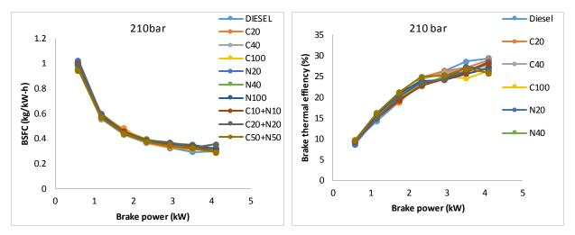
Fig 5. Variation of BSFC with BP for different blends (IP 210 bar)
