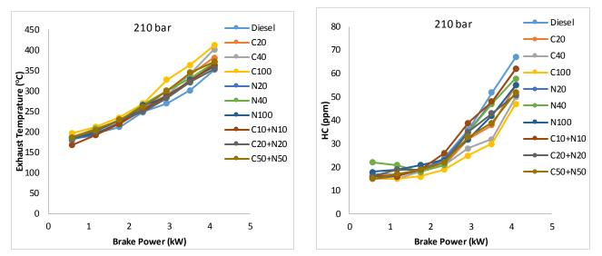
Fig 7. Variation of EGT with BP for different blends (IP 210 bar)
