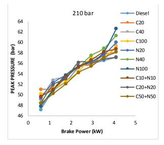
Fig 11. Variation of Peak pressure with BP for different blends (IP 210 bar)
