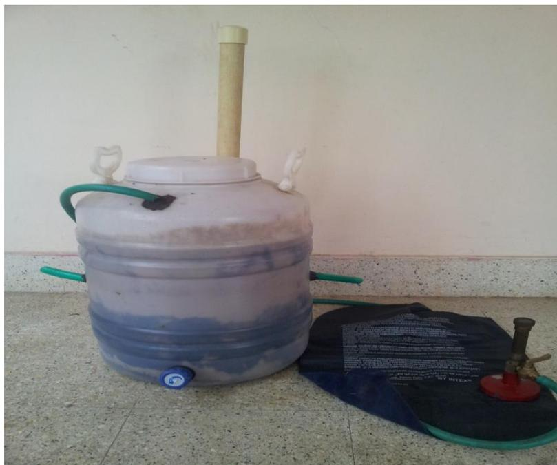
Fig. 2 Portable Biodigester
