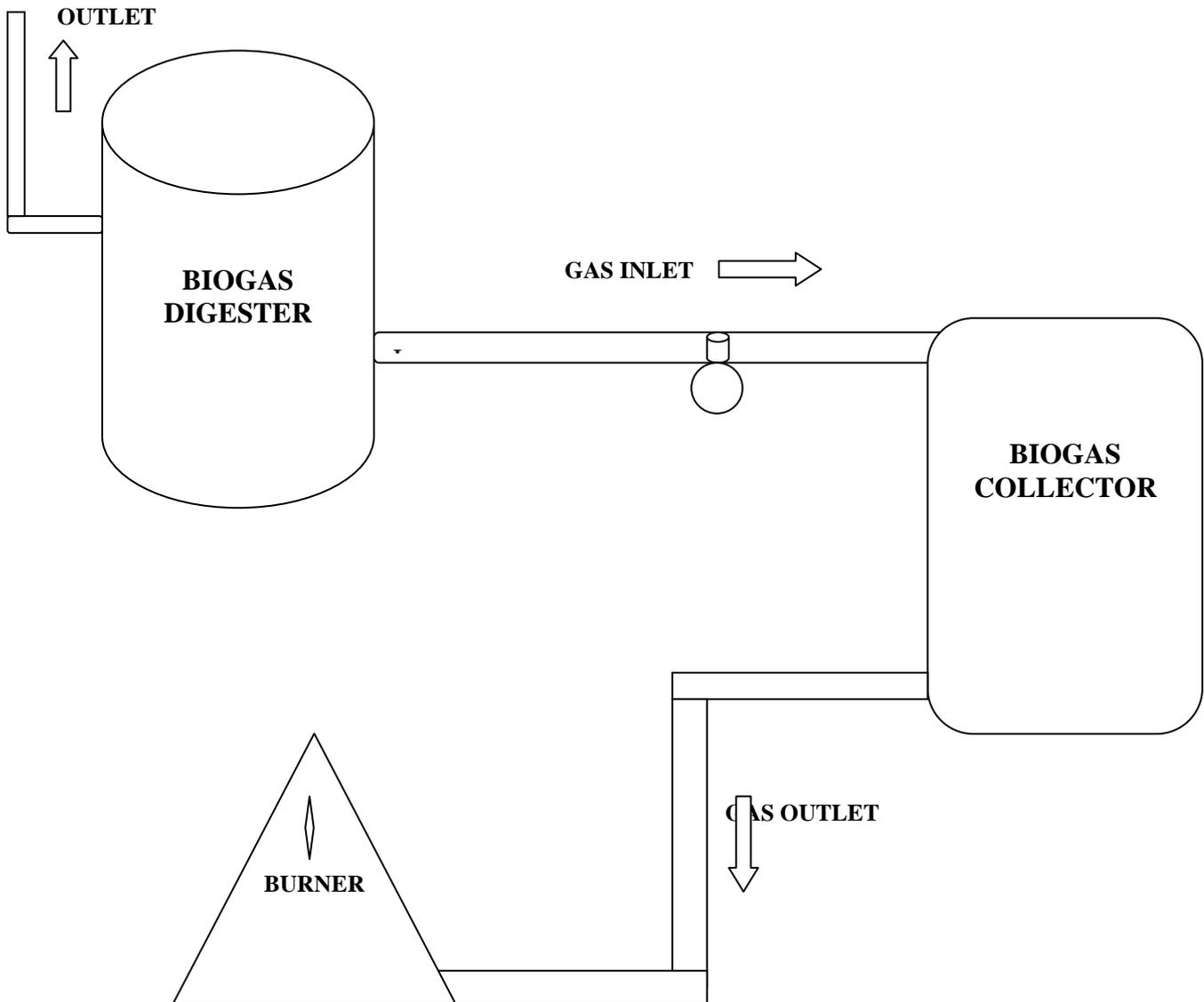
Fig. 1 Block Diagram of the Biodigester
