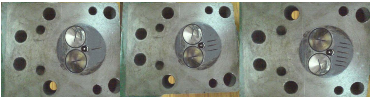
Plate1.Cylinder Head with a Single Channel, Three Channels and Six Channels.
