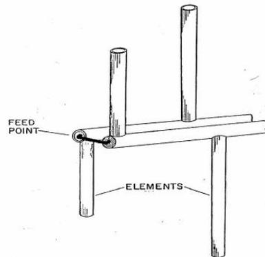
**Figure 5: Energizing dipoles by using coaxial line**
