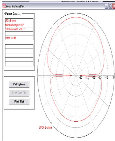
Figure 13: E-Plane pattern at 6 GHz
