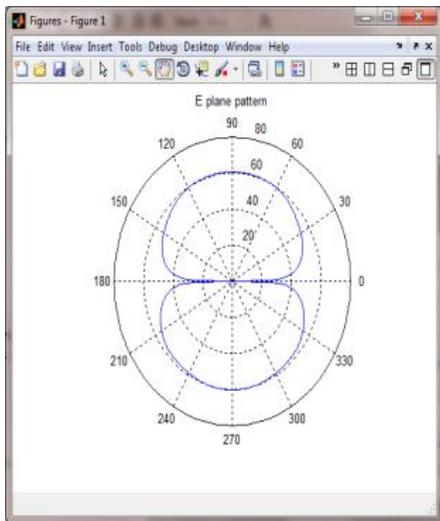
**Figure 7: E-Plane pattern at 0.5GHz**
