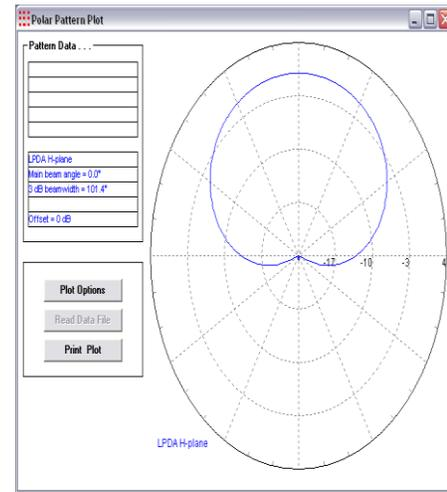
Figure 14: H-Plane pattern at 6 GHz
