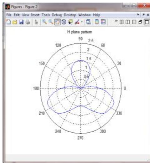
**Figure 8: H-Plane pattern at 0.5GHz**
