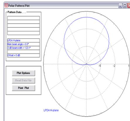
**Figure 12: H-Plane pattern at 0.5 GHz**
