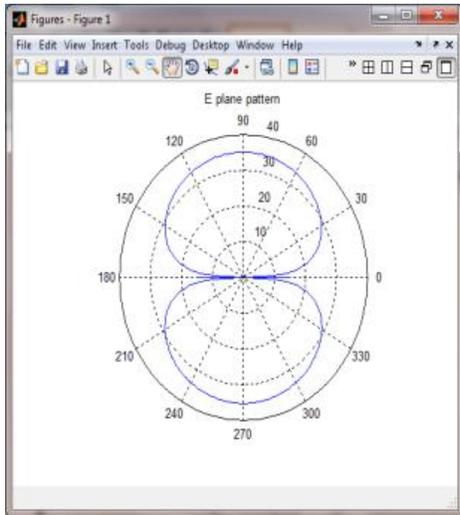
**Figure 9: E-Plane pattern at 6 GHz**
