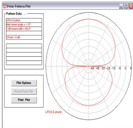
**Figure 11: E-Plane pattern at 0.5 GHz**
