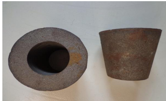
Fig.5 Bowl with Base material cast iron (nodular graphite)
