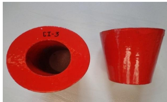
Fig.6 Bowl with Base material cast iron (nodular graphite) and Viscoelastic damping coating
