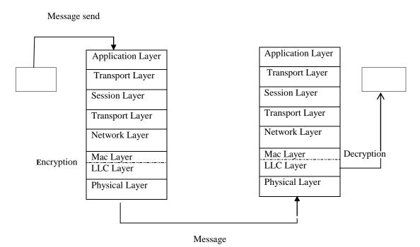
Fig 3: Encryption and decryption process between client and server
