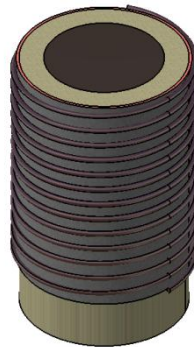
Figure 3. Thermal model of the induction furnace without the ceramic wall and with induction coil
