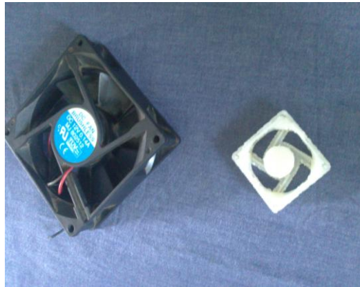
FIG 4.4.1 Prototype of miniaturized fan casing
