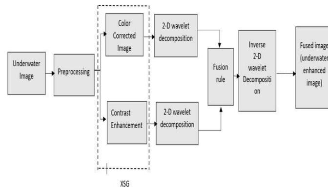
Fig.1 proposed block diagram of underwater image enhancement by wavelet decomposition
