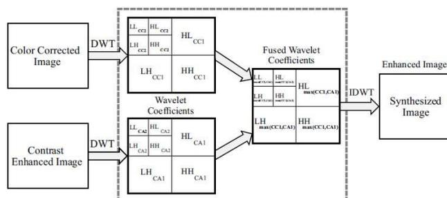
Figure 3: Two-level-2D decomposition, fusion of coefficients and image synthesizing
