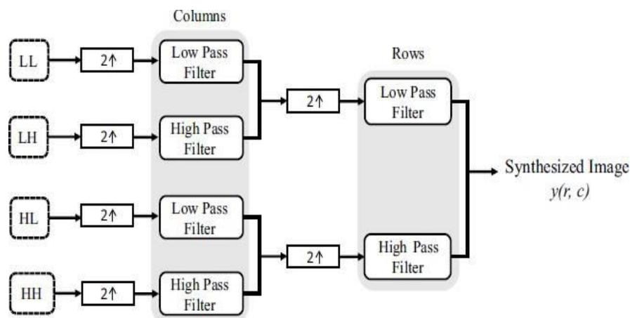
Figure 2:- One-level-2D wavelet-based inverse composition
