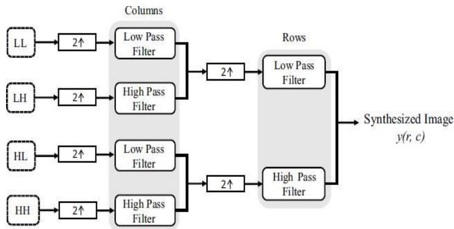
Figure 2:- One-level-2D wavelet-based inverse composition
