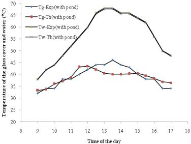
Fig.9. Theoretical and experimental values of average glass cover and basin water with coupled shallow solar pond
