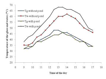
Fig.4. Variations of average glass cover and water temperature with and without shallow solar pond for the experimental days.
