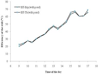
Fig.11. Theoretical and experimental efficiency of the solar still coupled with solar pond
