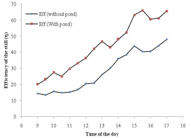
Fig.8. Comparison of efficiency of the solar still before coupled and after coupled with shallow solar pond
