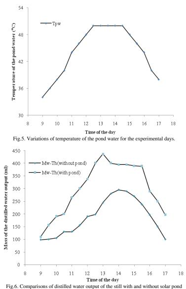
Comparison of efficiency of the solar still with and without integration of solar pond is depicted in Fig 8. It is found that the instantaneous efficiency of the solar still with solar pond is found to be higher than the efficiency of solar still without solar pond. The maximum instantaneous efficiency for the solar still without solar pond is found to be 48% and for solar still with solar pond is found to be 65% respectively.
