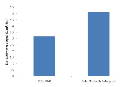
Fig.7. Comparisons of distilled water output in liters of still coupled with and without solar pond.
