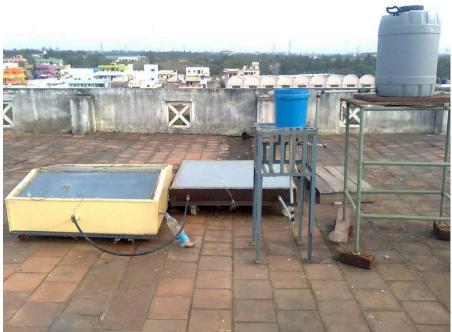
Fig.2. Photograph of the single basin double slope solar still integrated with shallow solar pond
