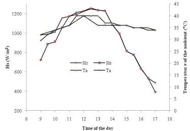
Fig.3. Variations of the solar radiation intensity and ambient temperature for one of the experimental days.
