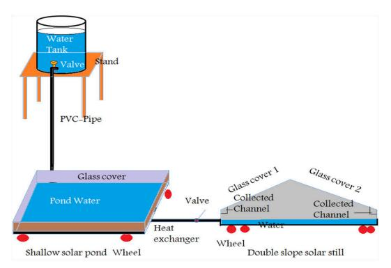
Fig.1. Schematic diagram of the single basin double slope solar still integrated with shallow solar pod
