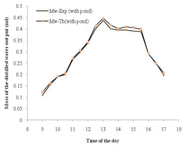
Fig.10. Theoretical and experimental values of distilled water output with coupled shallow solar pond
