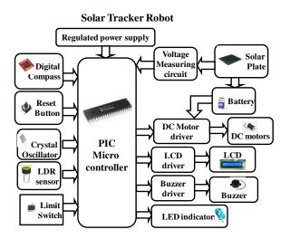
Fig.1 Architecture of solar robot tracking
