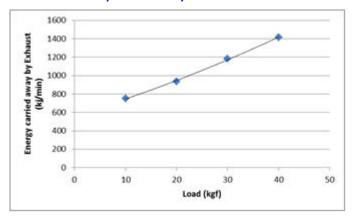
Fig.1.13 Variation of Exhaust energy with load at 2500 rpm engine speed
