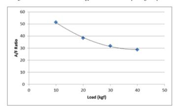
Fig. 1.14 Variation of A/F ratio with engine load at 2500 rpm engine speed
