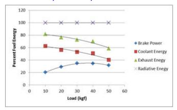
Fig 1.15: Percent fuel energy distribution at variable load and constant speed at 1500 rpm
