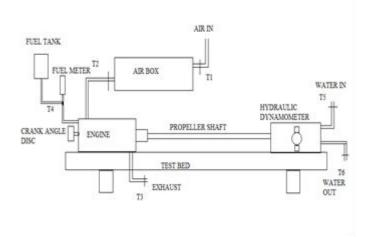
Fig. 1.1 Schematic Diagram of Diesel Engine Test Bed
