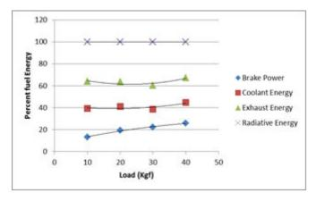
Fig 1.16: Percent fuel energy distribution at variable loadand constant speed at 2500 rpm
