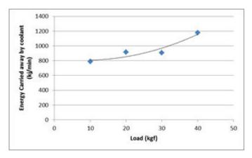
Fig 1.12 Variation of energy carried away by coolant with load at 1500 rpm engine speed
