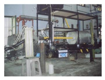
Fig. 1.2 HSDI diesel engine test bed
