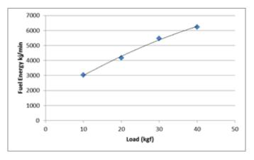
Fig 1.11 Variation of fuel energy with load at 2500 rpm engine speed
