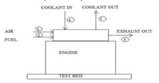
Fig. 1.6 Location of different temperatures indicators
