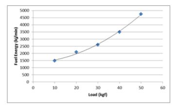
Fig 1.7 Variation of fuel energy with load at 1500 rpm engine speed
