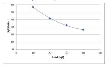
Fig 1.10 Variation of A/F ratio with engine load at 1500 rpm engine speed
