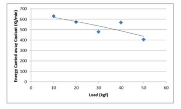
Fig 1.9 Variation of energy carried away by coolant with load at 1500 rpm engine speed
