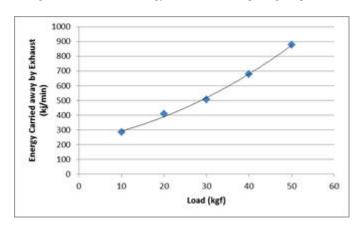
Fig 1.8 Variation of Exhaust energy with load at 1500 rpm engine speed
