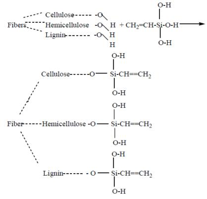
Fig. 3. Hypothetical reaction of fiber and silane. Reprinted with permission from Kalia, S. et al. [16].
