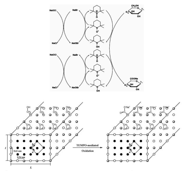
• Inaccessible glucose unit at core crystal Fig 5. Scheme of TEMPO-mediated oxidation mechanism of the hydroxymethyl groups of cellulose (top, reaction scheme) and crosssectional representation of cellulose nanocrystal indicating the occurrence of the surface TEMPO-mediated oxidation of available hydroxyl groups (bottom, surface crystal representations). Reprinted with permission from the Reference [6]. Copyright 2010, American Chemical Society)
