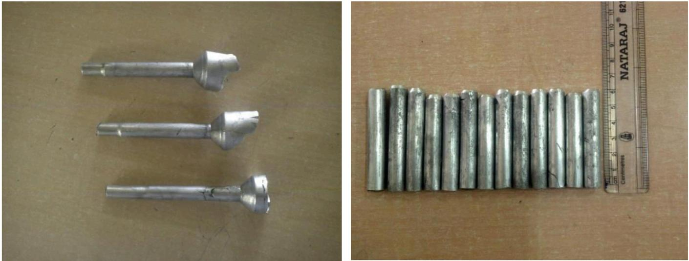
Fig 5. Compacted and Sintered specimens are subjected to hot extrusion (a) After extrusion (b) After removing the flash
